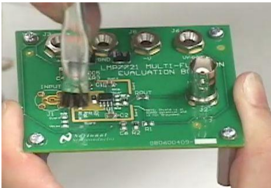
Figure 7: Cleaning board with Acid Brush
